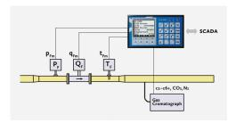
Natural gas flow measurement with ultrasonic meter
