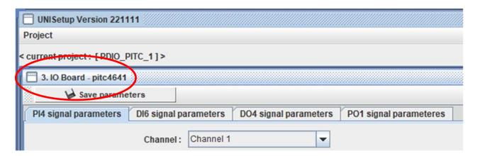
Existing parameter projects with PDIO484 board parameters will also work with the PITC4641 board without any modification.
