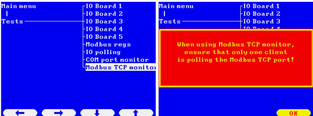
Ensure that only one Client polling the Modbus TCP port. Generally, it is allowed to poll the Modbus TCP port with several Clients. In case of Modbus TCP monitoring temporary disable the polling from all but one Client. Press OK to acknowledge the warning message.
