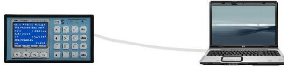
Flow computer – PC Ethernet direct connection
