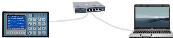
Flow computer – PC Ethernet connection using switch
