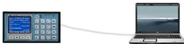
Flow computer – PC Ethernet direct connection
