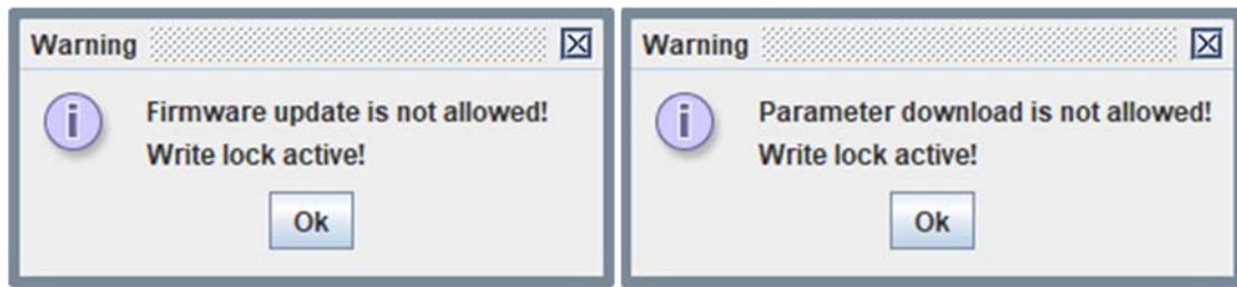
Figure 6-9 Write lock message on ToolBox
