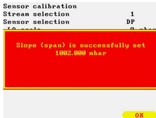
Figure 9-178 DP sensor slope calibration finished display
