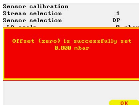
Figure 9-176 DP sensor offset calibration finished display
