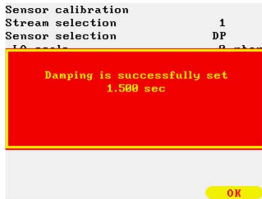
Figure 9-180 DP sensor damping finished display
