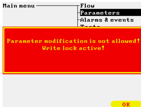
Figure 6-8 Write lock message on display
