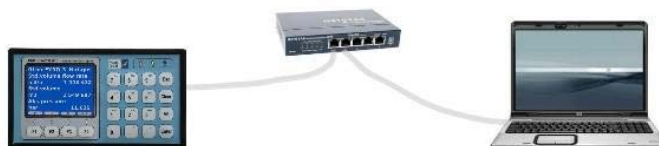
Flow computer – PC Ethernet connection using switch
