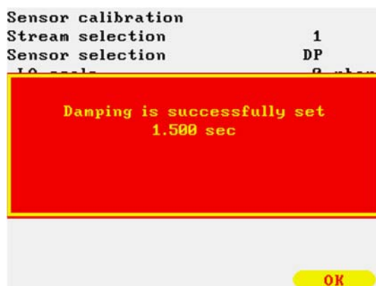
Figure 9-180 DP sensor damping finished display
