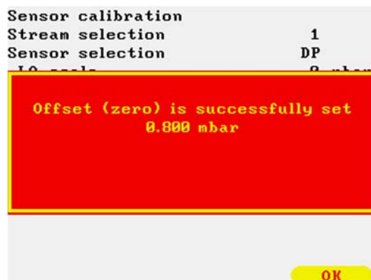
Figure 9-176 DP sensor offset calibration finished display
