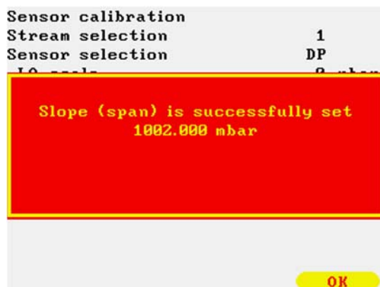
Figure 9-178 DP sensor slope calibration finished display
