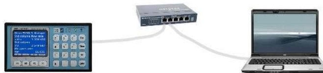
Flow computer – PC Ethernet connection using switch
